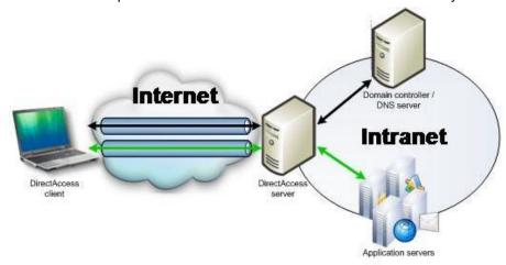
Figure 1 DirectAccess clients access the intranet using IPv6 and IPsec
